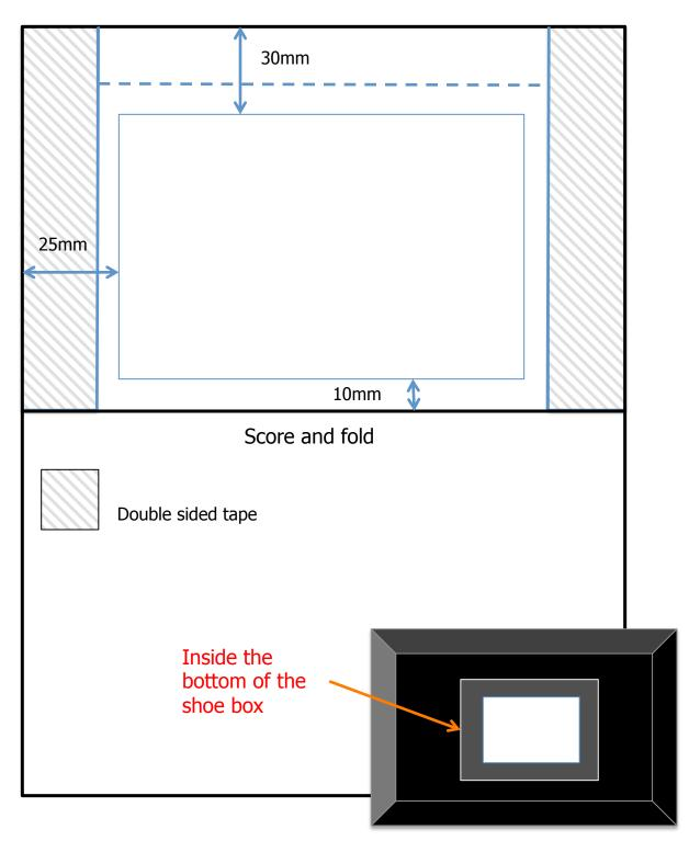
6. Next we have to load the photo paper. Above is the template for the photographic paper holder, using A4 black card. This attaches inside the bottom of the shoe box using Velcro.
