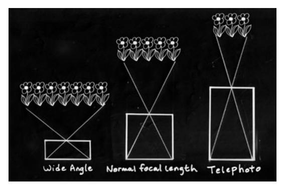
A focal length about equal length to the diagonal size of the paper or film is a normal focal length. A shorter focal length is called a wide-angle, and a significantly longer is referred to as telephoto.
