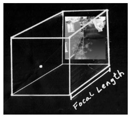
The focal length of your pinhole camera is the distance between the pinhole and the paper you have loaded the camera with.
