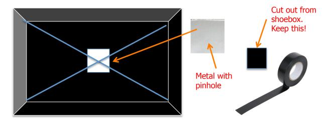
5. Make the shutter. Using a beer mat, tape over the pinhole and secure with velcro (stick the discarded square to completely block out the sunlight).
